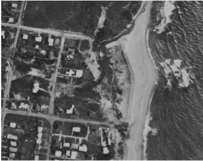
Figure 7: Imagery from the then Beach Protection Authority indicated dune severe sea erosion between 1972 to 1974 and damage to the January 1974 reconstructed dune above.
