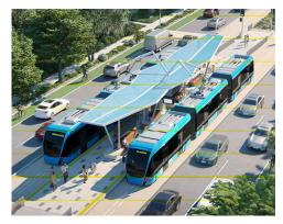
The same in every respect as the Light Rail Transit system but powered by on board batteries so there are no overhead wires.
