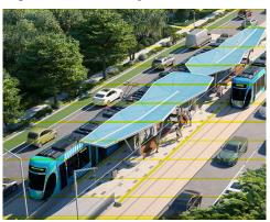
Carries up to 300 passengers, replacing up to 250 cars, and offering a very high-quality ride, running on steel wheels and tracks in the pavement and powered from overhead wires.
