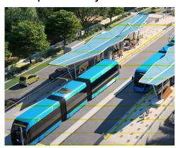
Carries up to 140 passengers, replacing up to 110 cars, and offering a reasonable quality of ride, running on tyres and powered by batteries, so there are no tracks in the pavement and no overhead wires.
